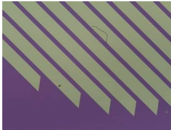
Figure 2-8 Low Stress Silicon Nitride Window on Silicon Support Structure Geometry
